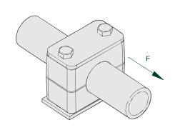
All tightening torques and maximum loads in pipe direction regard clamps with upper plates and hexagon head bolts according to EN ISO 4014/4017.
